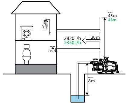
**GB** Self-priming gardening pump, also suitable for the pressurisation of water in domestic applications. Compact, light, robust and easy to use. Equipped with orientable connections plus integrated non-return valve and pre-filter for extended pump life. Facility to empty residual water to protect it from frost and accumulation of limescale also included.
