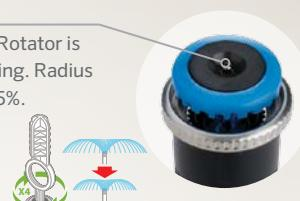
**Arc Adjustment Ring** Install the MP Rotator with the Left Edge Indicator aligned with the left edge of the landscape. The MP Rotator not only features a fully adjustable arc, but as the arc is changed, the flow adjusts proportionally to maintain matched precipitation.
